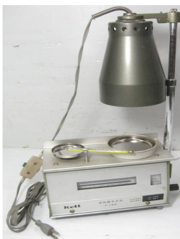
Fig. 4. Moisture analyzer “Kett Electric Laboratory”, made by “Infrared Moisture Meter Model F-IA”
