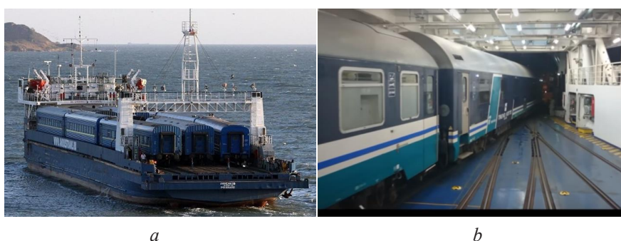
Fig. 1. Transportation of passenger cars on rail ferries by sea: a – “Annenkov” ferry (Sea of Azov); b – Fata Morgana ferry (Strait of Messina)
