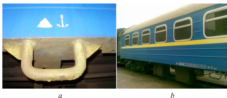
Fig. 2. Staples for fixing the passenger car body relative to the deck: a – fastening to the car body; b – placement along the car
