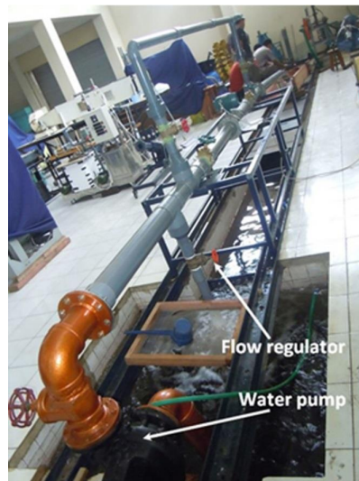
Fig. 5. Water Flow Rate Regulator
