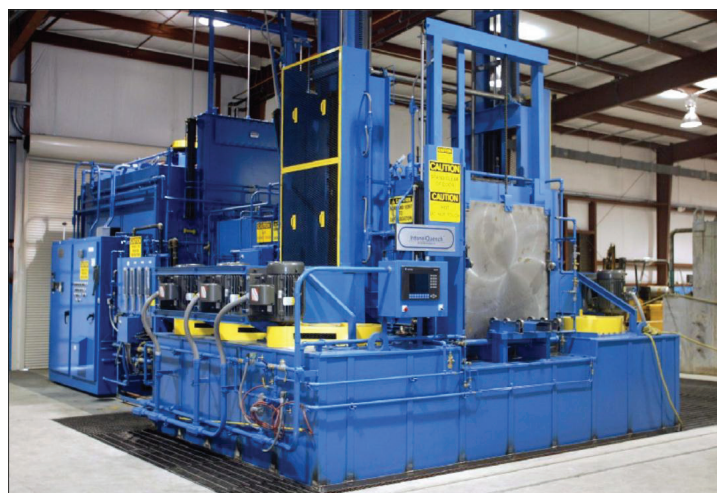
Fig. 2. Integral quench atmosphere furnace equipped with 41 m 3 IQ water tank built by AFC-Holcroft and installed at Euclid heat treating Co
