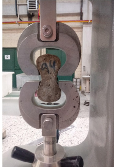
Fig. 5. Apply tensile strength to specimens
