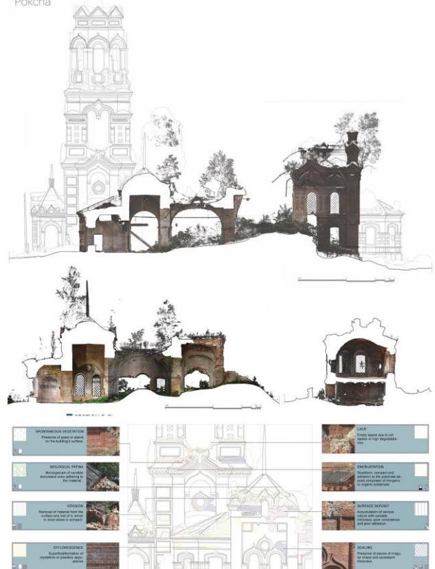
Figure 6. Point cloud views and drawings with analysis of the decay of the Church of Annunciation.
