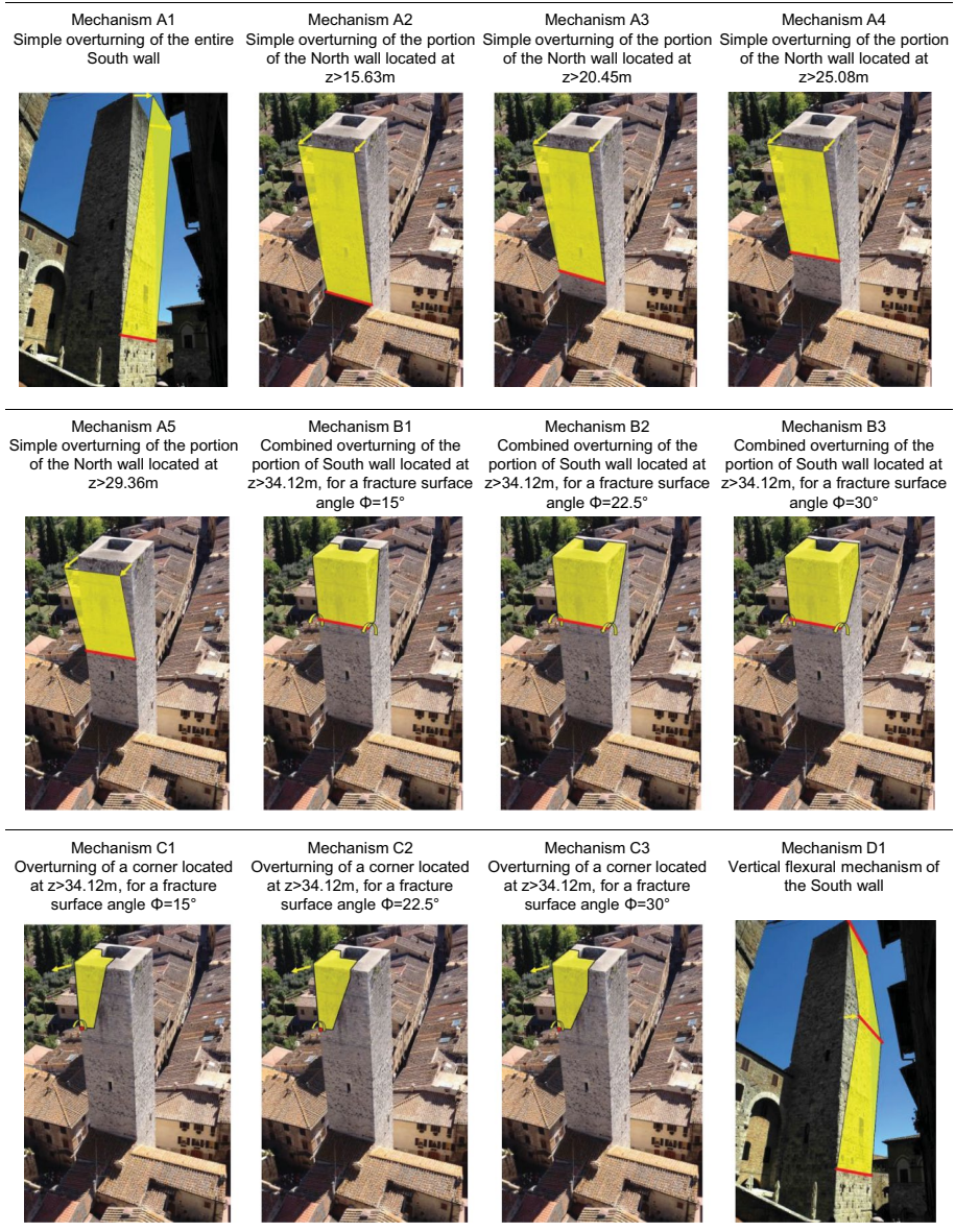
Fig. 7 Considered failure mechanisms
