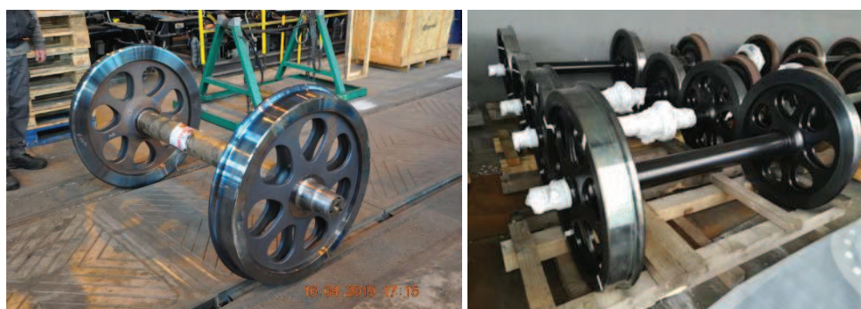
Fig. 5 Left: the first Liberty Wheel produced. Right: set of wheelsets ready for line tests (one conventional bogie and one with Liberty Wheels for comparison).
