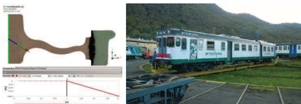
Fig. 3 Left: Finite Element proved that the solution without retaining ring is as safe as the one with the retaining ring. Right: during the line tests (Nov. 2018).
