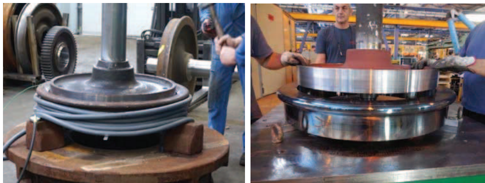
Fig. 2 Left: Tyre removal by means of a portable induction heating device. Right: tyre fitting without retaining ring
