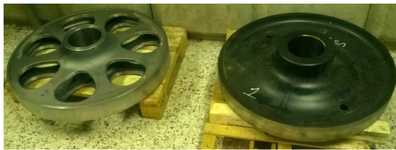
Figure 14 Top: the very first wheelset with Liberty Wheels (16.04.2019). Bottom: comparison of the Liberty Wheel with the original wheel centre
