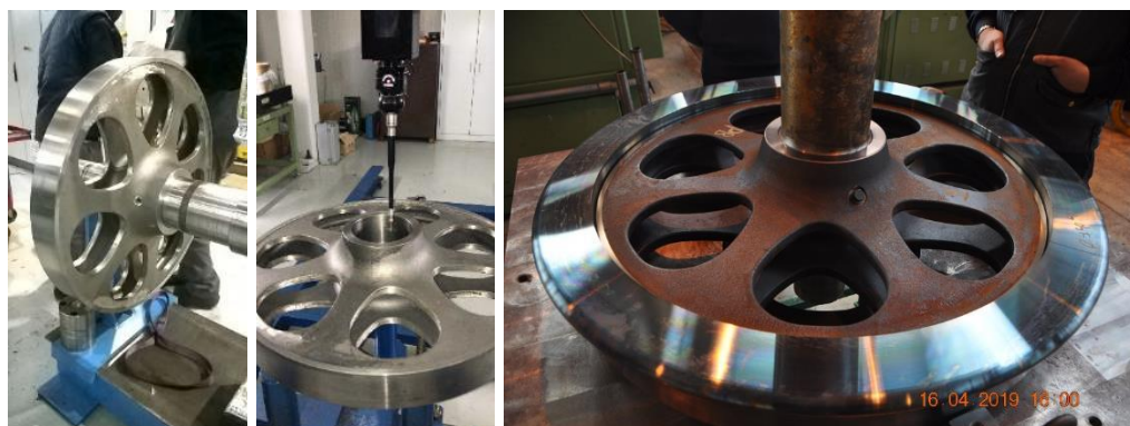
Figure 13. Left: first mounting on an axle. Mid: CMM dimensional check. Right: first Liberty Wheel assembly with the tyre.
