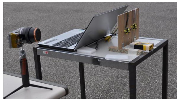
Figure 5: infrared camera, PC, sensors and laser measuring: positions for the test
