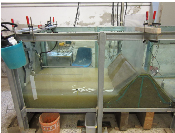
Fig. 3 Constructed model levee at DICEA (Department of Civil and Environmental Engineering, University of Florence) 48 h after release of crayfish into the setup
