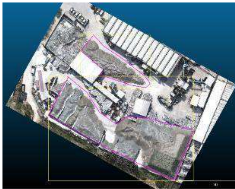
Figure 25. Stockpiles compared with CloudCompare software.
