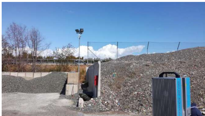
Figure 2. Laser scanner survey of the waste stockpile.
