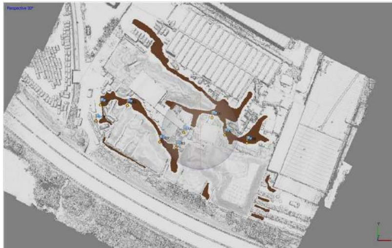
Figure 17. Manual classification of the ground in Photoscan for generating the DEM reference base.
