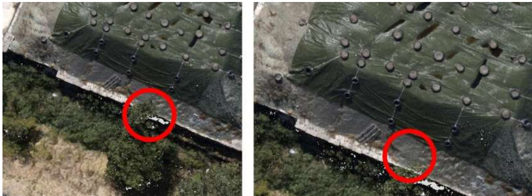
Figure 16. Dense cloud cleaning before DEM generation.
