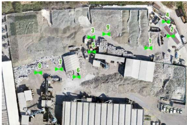
Figure 10. The survey area and the position of targets used as GCPs and CPs.
