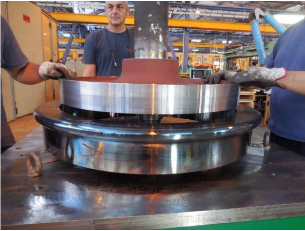
Fig. 6 Lowering a trailed wheelset on a hot tyre resting on the specifically designed mounting jig with calibrated shims.
