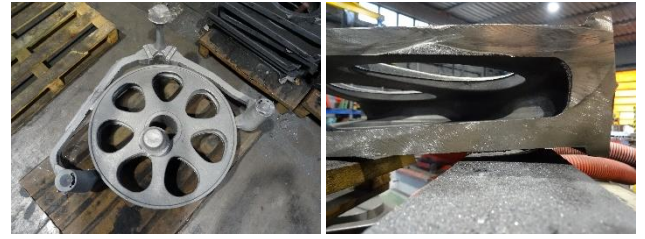
Fig. 3 Final casting after sanding (left) and cut wheel centre to obtain specimens for destructive tests (right).
