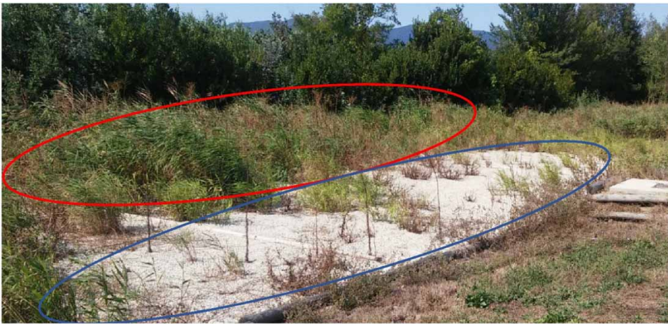
Figure 3 | Example of uneven growth of P. australis in horizontal tank, line B of the CW: in red circle good growth of plants due to good irrigation with the influent and in blue circle poor/absence of growth. Please refer to the online version of this paper to see this figure in colour: http://dx.doi.org/10.2166/wst.2019.030 .
