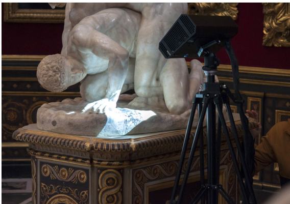
Figure 4: 3D scanner and its projected light that bounces on the artwork.
