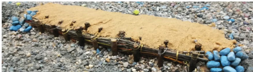
Fig.2A fascine with ripraps upstream and downstream
