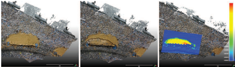
Fig.4 Example of diachronic analysis a) before the run, b) after the run, and c) difference The color scale varies from blue (absence of erosion) to red (maximum erosion).
