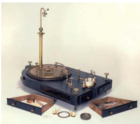
Figure 2b. One of the original astatic galvanometers, built by L. Nobili in 1826 and preserved at the "Museo Galileo," the museum of the History of Science, in Florence, which owns several of Nobili's devices.
