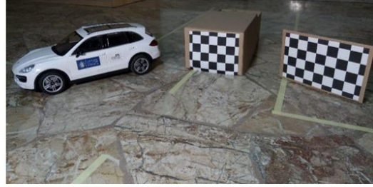
Figure 2. The five elements used for the generation of the dataset: a stereo camera, a scaled model of a real car, a moving box sized as the scaled car, a scaled model of an intersection of streets, and two checkerboards.
