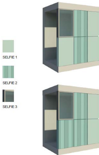
Figure 7. Selfie_3: a. Glass layer with PVB and IR reflecting coatings; b. Air gap and shading device; c. double glazing
