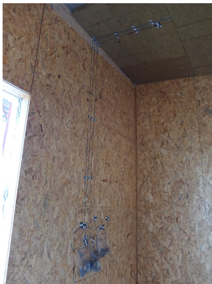
Figure 17 – Probes installation in the roof layers
