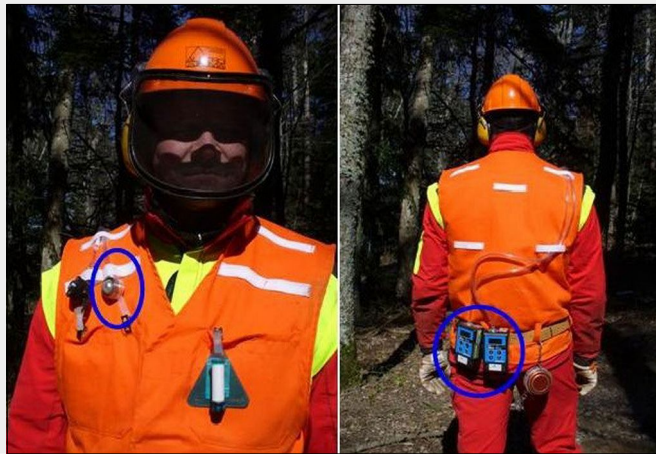
Fig. 1 - Personal sampler. SKC Button Sampler on the operator's jacket (left) and Gilian 5000 portable pumps (right).
