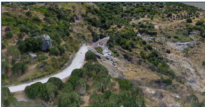
Figure 5. 3D view of the ortho-photo acquired at the Scillato landslide projected over the DTM generated from the point cloud. The damage generated by the slope movements to the local road is clearly visible on the image.
