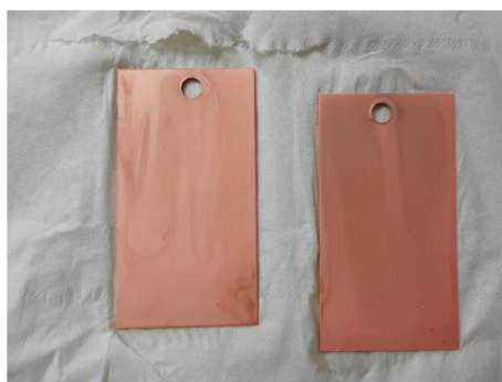
Fig. 1. Cu-coated samples for current density 3.45 \text{A dm}^{-2} , deposition time 1 min.
