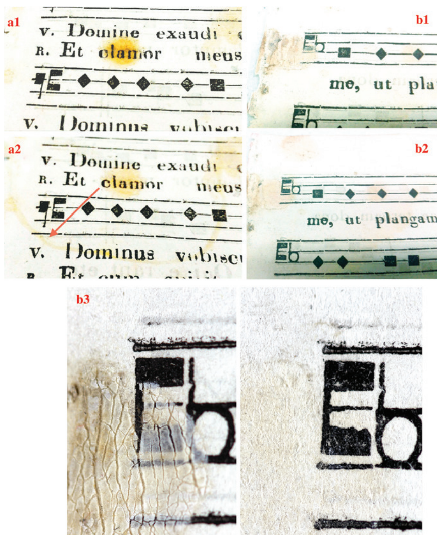
Fig. 8: (a1–2) Application of the PMMA-MEK organogel previously developed for the cleaning of painted canvas. (a1) Wax spot before cleaning. (a2) After the application and removal of the less retentive gel, a tideline has formed owing to the uncontrolled spreading of the solvent, which migrated carrying dissolved wax. (b1–3) Application of the new PMMA-MEK.3 gel. (b1) Wax spot before cleaning. (b2) The same area after the application of the gel. No tideline is observable, thanks to the improved retentiveness of the gel as compared to the previous formulation. (b3) Detail of the cleaning intervention showing the presence of wax before the removal (left) and the inked paper after removal of wax using the PMMA-MEK.3 organogel (right).
