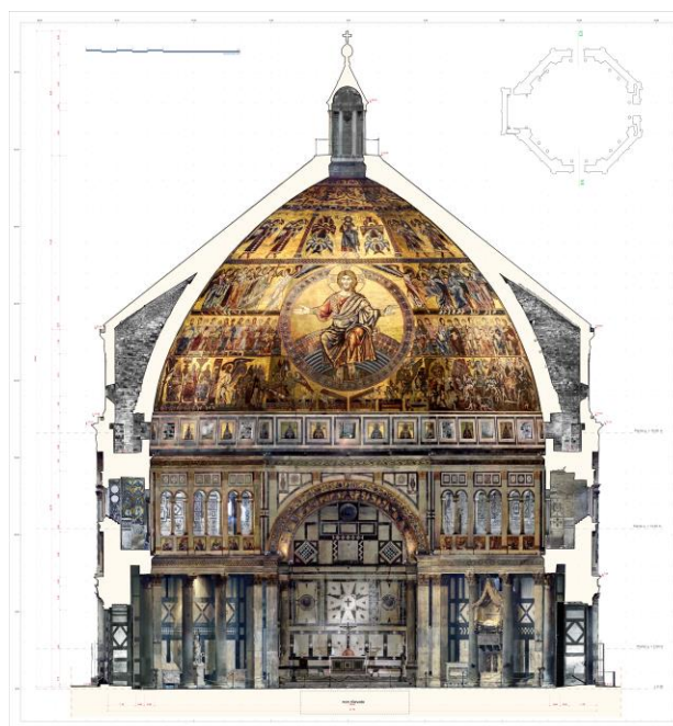
Figure 4. Longitudinal section: vectorial drawing and orthoimage
