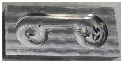
Fig. 9 Specimen machined with the archetype toolpath.
