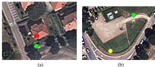
Fig. 1. a) Outdoor-to-Indoor scenario. The green and red circles represent the aiding GPS receiver located outdoor and the indoor aided one, respectively. b) Outdoor-to-Outdoor scenario. Both the aiding (green circle) and the aided (yellow circle) receivers are located outdoor.
