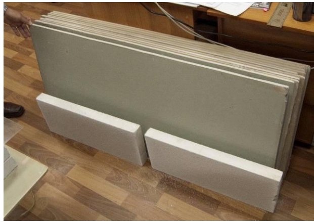
Fig. 6. Photograph of ten plaster sheets (in the background) and two foam bricks that were used in experiments.
