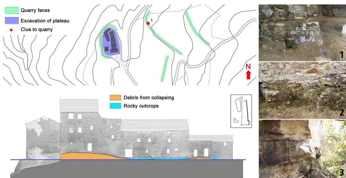
Fig. 9 – The geological analysis allowed to verify that the material with which the whole town was built comes from the same geological area, so it seemed logical to look for a possible quarry in the vicinity of the castle: 1. Internal masonry on rocky outcrop, 2. Outcrops on East side of the settlement, 3. Metric verification of the origin of the stones (S. Di Grazia)
