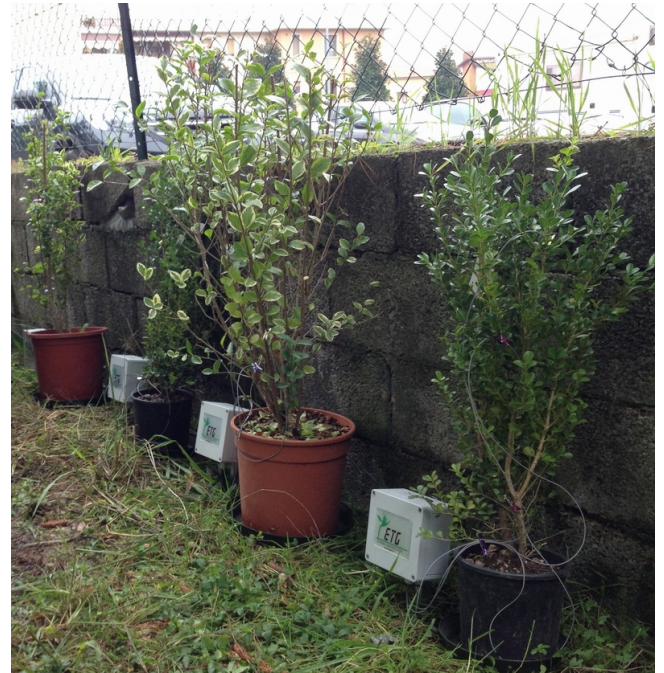
Fig. 2. The deployed ligustrum and buxus plants as biosensors.
