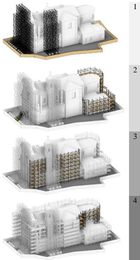
Figure 2. Sample installation of the scaffolding
