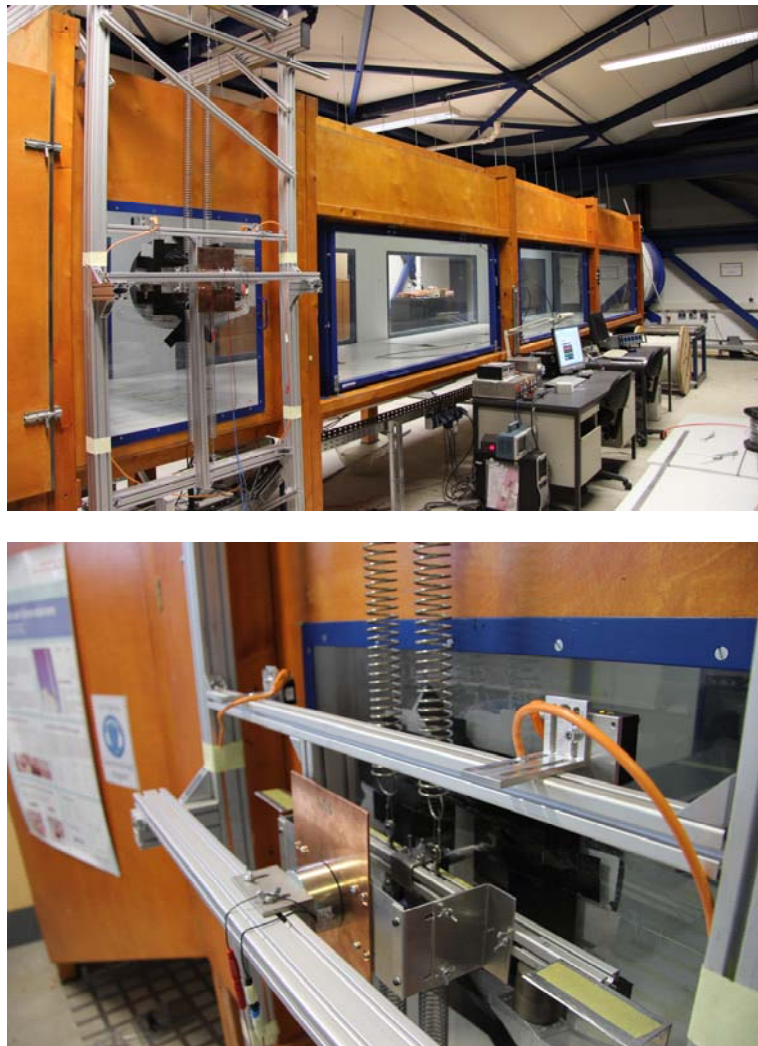
Figure 2. View of the wind tunnel facility from the inlet side (top) and detail of the aeroelastic setup, showing the measuring apparatus and electromagnetic dampers (bottom).
