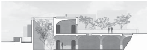
Figure 5. Square with basement parking: section (Dissertations 1 ).
