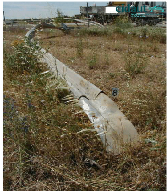
Figure 14: Result of an impact involving the first few posts of a terminal [1]
