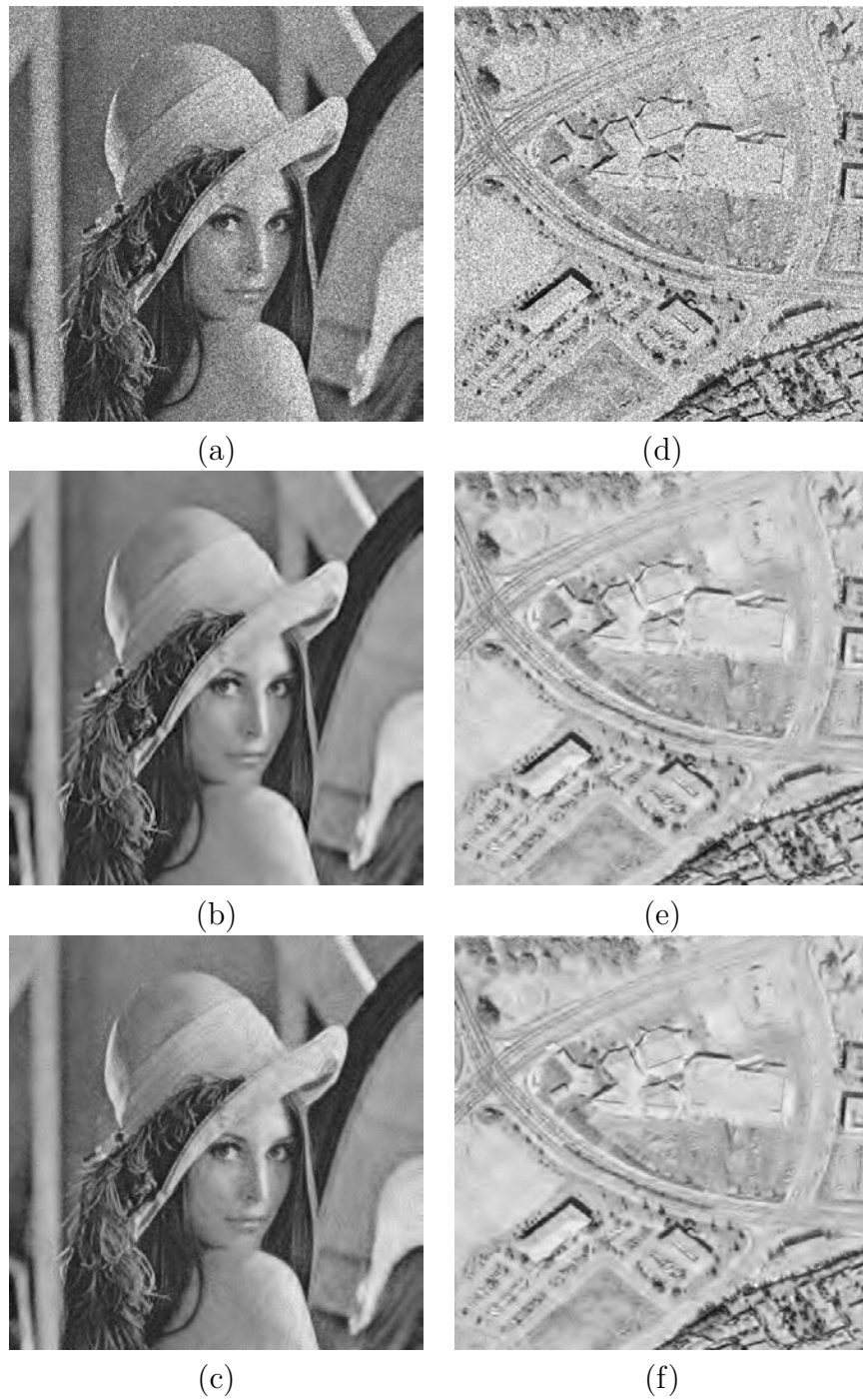
Figure 3.9: Results obtained with the test images Lena (a)-(c) and Aerial (d)-(f) degraded with 4-look speckle: noisy images (top); the best (middle) and the worst results (bottom) achieved according to Tables 3.2 and 3.5.
