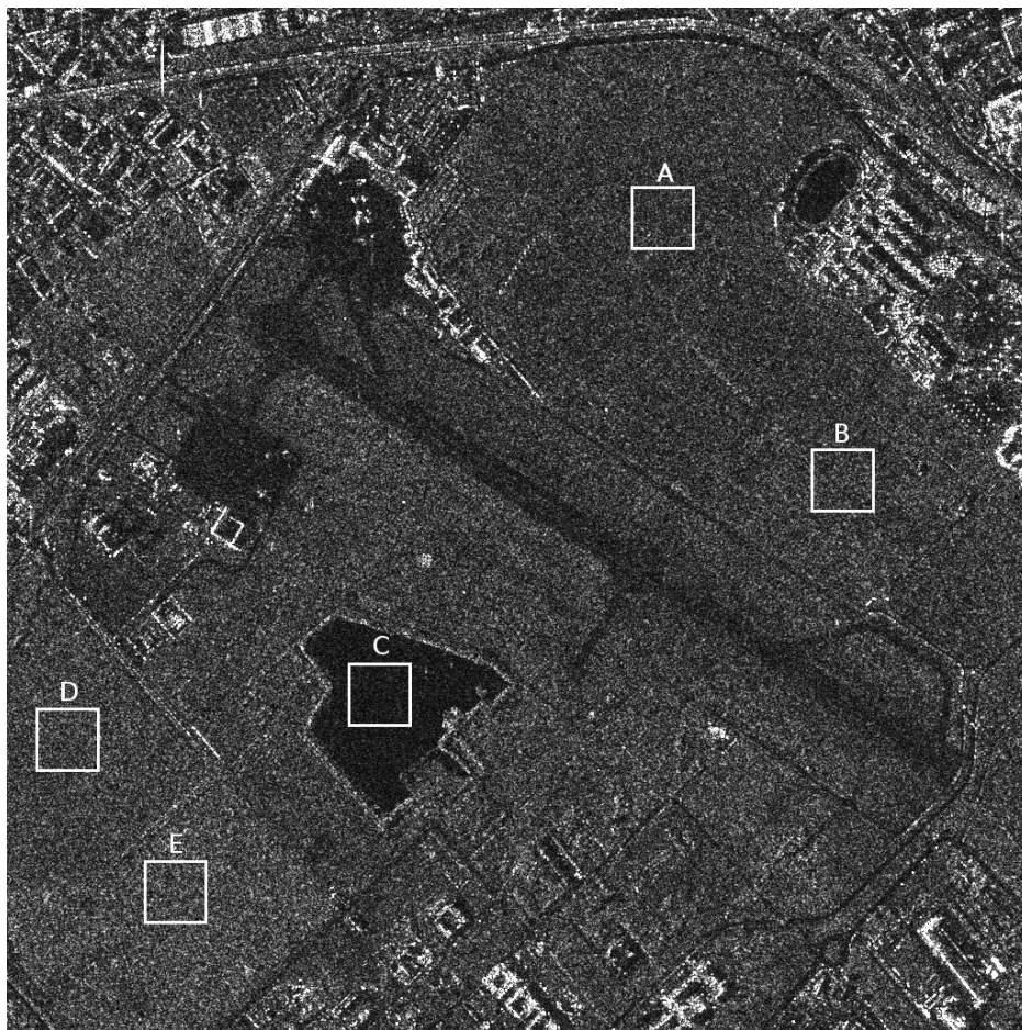
Figure 3.10: Original COSMO-SkyMed image ( 1024 \times 1024 , 3m resolution): five homogeneous areas are denoted with capital letters and used for ENL estimation.
