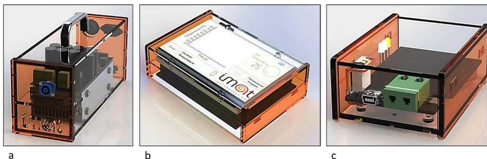
Fig. 13. The IMAT components: a - The IMAT power box, here rendered, is subdivided in its mains components: the IMAT Main Board and the AC/DC Switching Power Supply which assures galvanic insulation of the output voltage; b - rendering of the IMAT Control Unit; c - rendering of the IMAT TC Unit.
