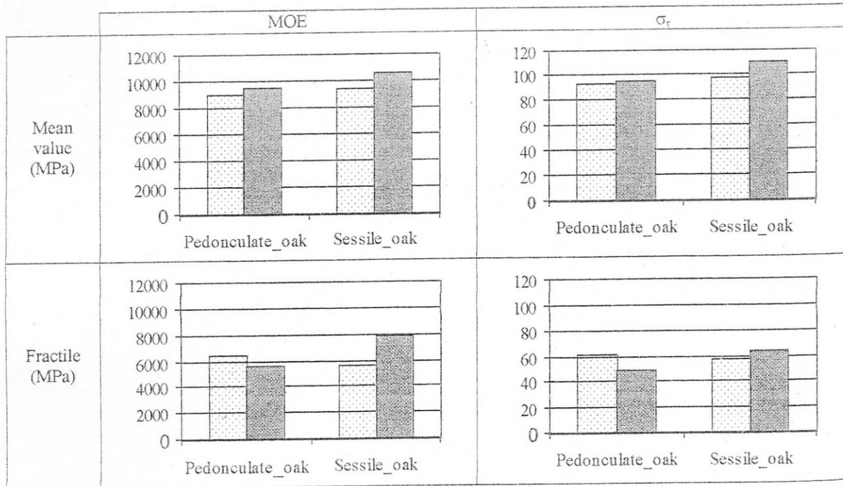
Figure 3 : Veneer thickness effect on oak LVL MOE, rupture stress mean values and fractile to 5% (all the data)
