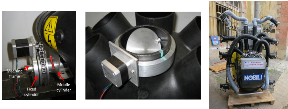
Fig. 6, 7, 8 : Fan air flow rate control, actuated by a mail butterfly valve; the variable inclination, step motor controlled.
