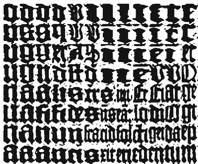
Fig. 7 Example of a 12 \times 8 SOM map. Each neuron is represented by the closest pattern belonging to the corresponding cluster
