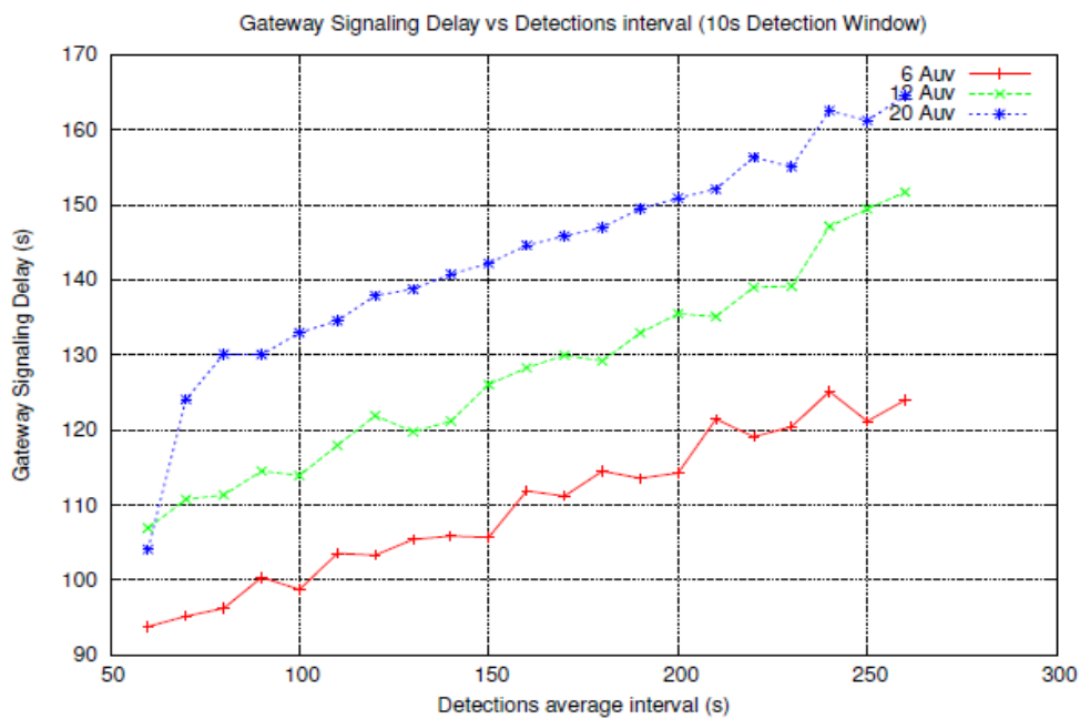
Figure 8. Average Surface Gateway signalling delay against detection interval, for different number of nodes.
