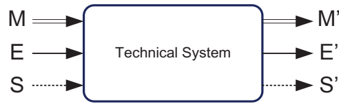
Figure 1: EMS model: Energy, Material and or Signals are channelled or converted to deliver a certain function.
