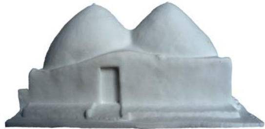
Figure 11. Solid model of dwelling units in the village of Er Raheb (Syria) – sinterized
