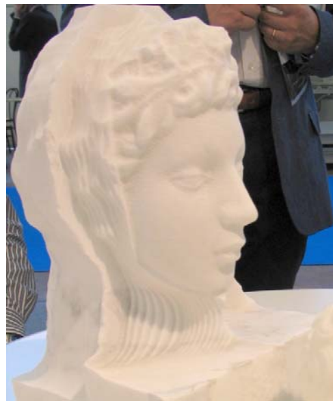
Figure 12: The marble replica of a statue's head at an intermediate working phase: subsequent step of machining are visible; the level of detail showed on the face is the last finishing obtained
