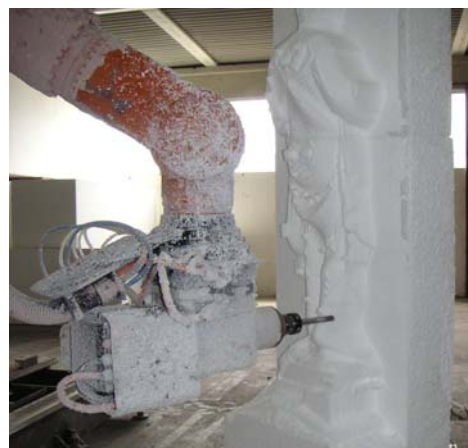
Figure 5. A CNC robotic milling machine working on the replica of the stature in Figure 2
