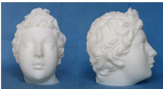
Figure 14. Real scale model of the head's statue shown in Fig. 2 – Fuse deposition model
