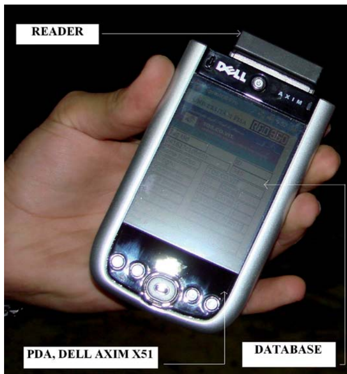
Fig. 2 - Palm-PC with reader for TAG identification.
