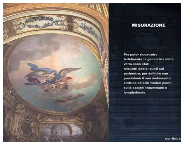
Figure 13 – A multimedial tool has been used to refer topographic measures. First form shows the vaulted ceiling.
