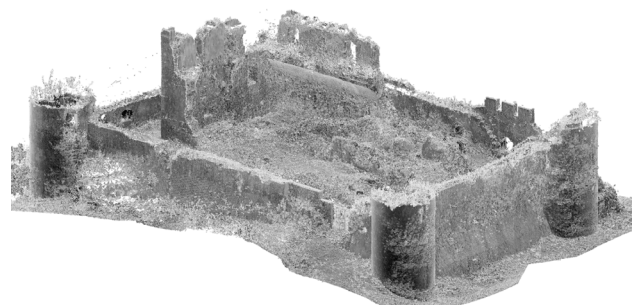
Figure 5. View of the points model surveyed using three-dimensional scanning
