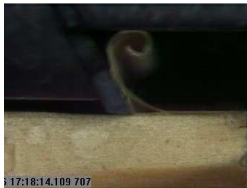
Figure 5. Douglas Fir processed at high speed with 0,2 mm of d.o.c.
