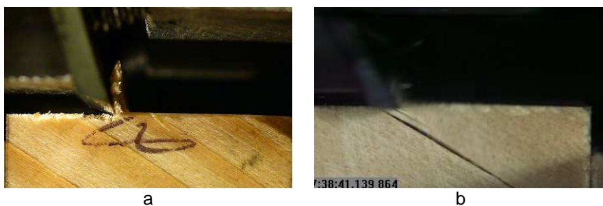
Figure 8. Douglas Fir processed at -30^\circ of grain angle with low (a) and high (b) speed with 0,2 mm d.o.c.
