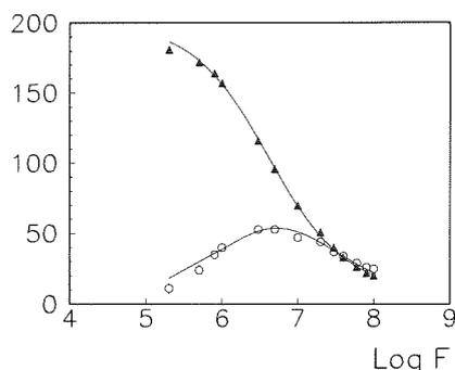
**Figure 3.** Measured and calculated complex permittivity versus frequency ( $F$  is frequency in hertz) for a PFPE W/O microemulsion with  $W/S = 0.3$  w/w and  $O/S = 1.71$  w/w. Triangles:  $\epsilon'$ ; circles:  $\epsilon''$ .
