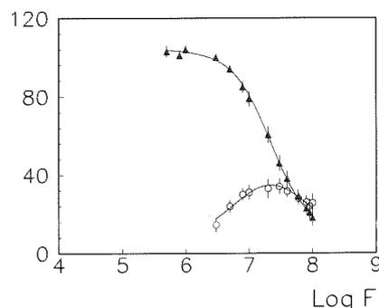
**Figure 4.** Measured and calculated complex permittivity versus frequency ( $F$  is frequency in hertz) for a PFPE W/O microemulsion with  $W/S = 0.3$  w/w and  $O/S = 0.87$  w/w. Triangles:  $\epsilon'$ ; circles:  $\epsilon''$ .
