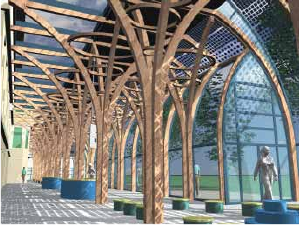
Figure 8 Meyer Hospital. The surface of the sunspace will incorporate a semi-transparent PV system with a rated capacity of 31 kWp of renewable energy. The Meyer's sunspace is orientated to the south.. Design strategies consider not only energy and environmental aspects but also social impacts: the primary objective is to create a pleasant "socializing" space that can be used through much of the year without requiring any extra energy. This social space is integrated with the green park. PV installation was financed by the Ministry of Environment after a national competition on "PV High Architectural Integration".
