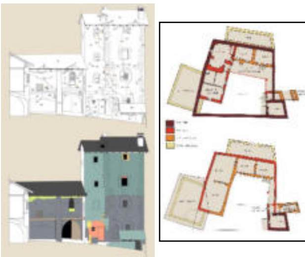
Figure 11. An example of stratigraphic survey on a facade; hypothesis of chronological reconstruction of the Povil Casaforte.
