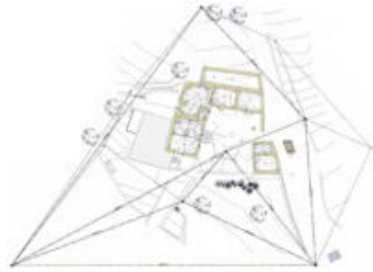
Figure 7. Topographic network and direct survey schema.
